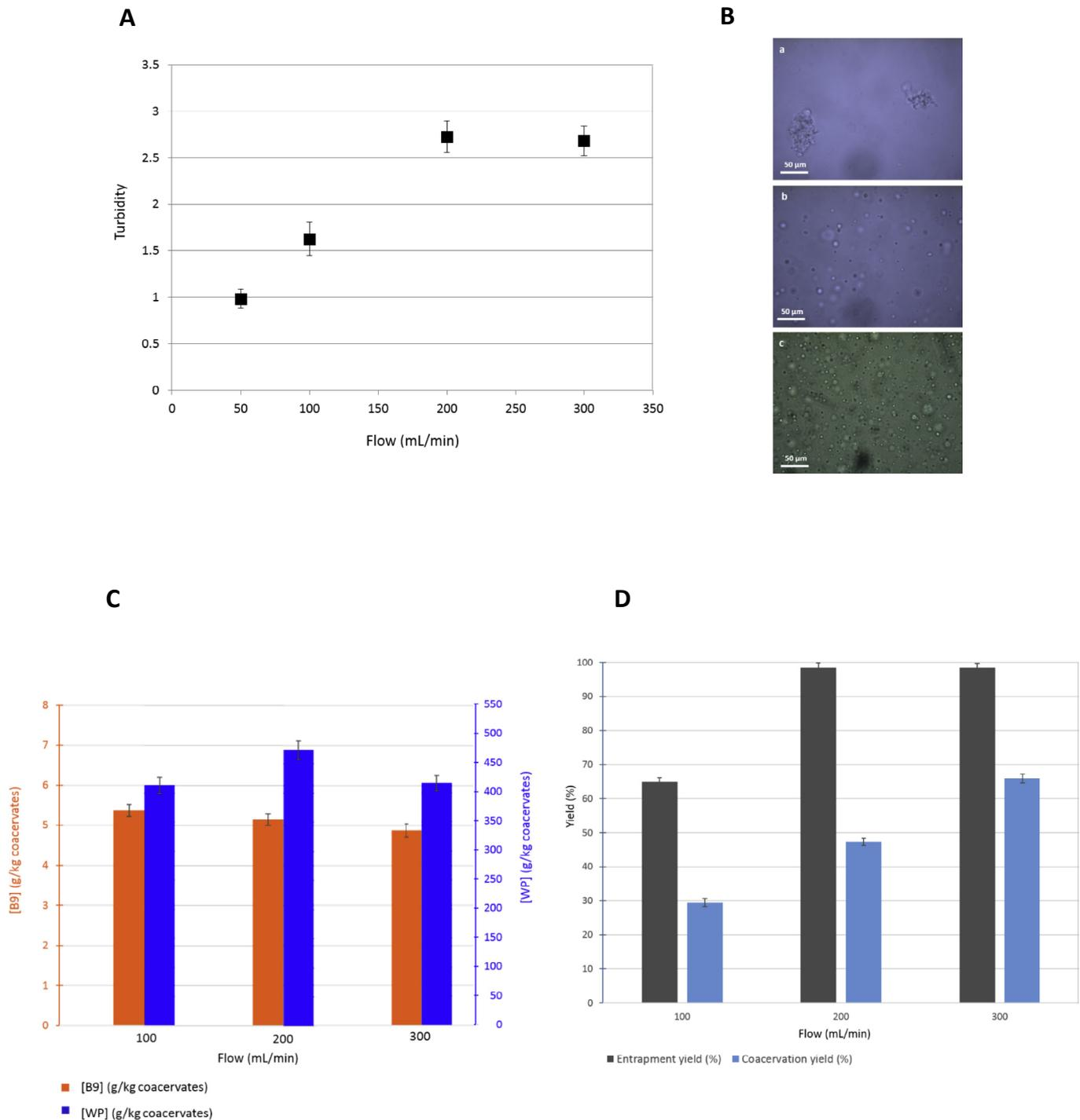
**Fig. 5.** Continuous coacervation of B9-WP depending on initial flows. **A:** Turbidity of B9-WP solutions measured at different initial flows (mL/min) through the static mixer, **B:** Corresponding particle morphology prior centrifugation: (a) flow = 50 mL/min, (b) flow = 100 mL/min, (c) flow > 200 mL/min, **C:** B9 and WP concentrations in B9-WP coacervates, **D:** Entrapment of B9 and coacervation yield after centrifugation.
